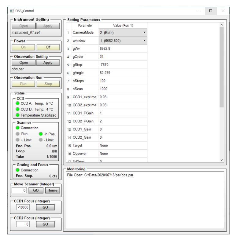
Focusing. Screen the some portion of slit and check wheter the boundary is clear in display. The second way is to check wheter the brightness in slit (y) direction varies ahrply in spectrogram. (It is quite useful to run the video focus mode to check the spectrogram and line profile simultaneously. Set the AcqMode equal to 0 (video mode) and then click the Apply button in Obseravtion Setting tab then click the run button in Observation Run tab.)
